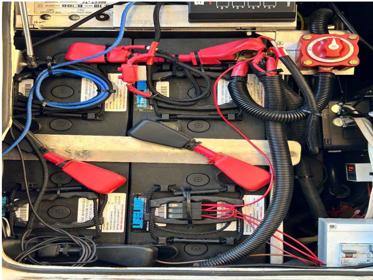
Figure 6 House AGM Battery Bank
