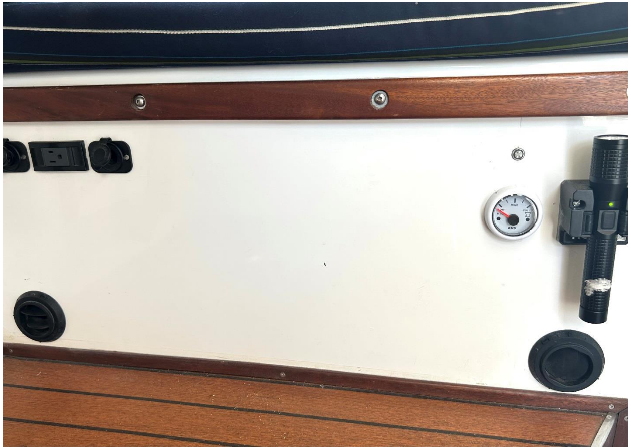
Figure 12 Dinette Outlets and Webasto Fuel Monitor
