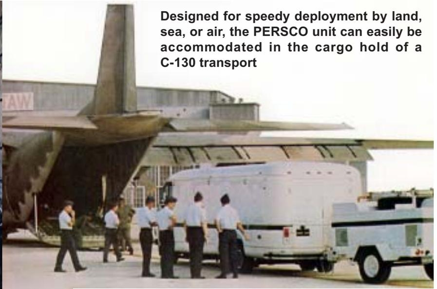
Designed for speedy deployment by land, sea, or air, the PERSCO unit can easily be accommodated in the cargo hold of a C-130 transport
