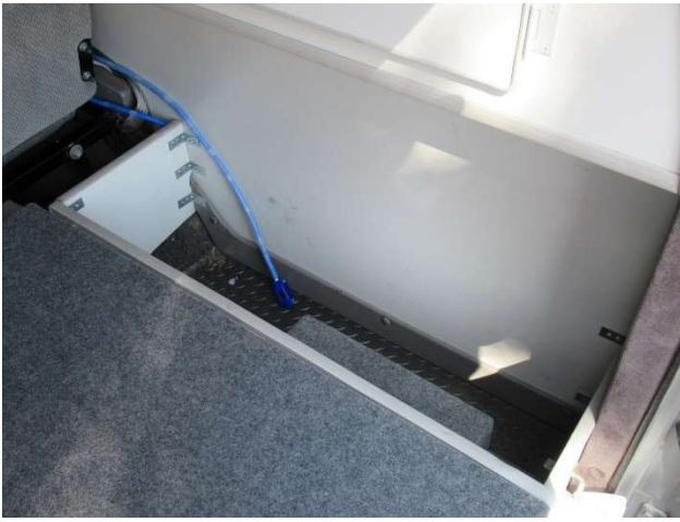
Interior rear storage: main compartment 40"Wx55"Dx13"H, and side cabinets 14"Wx36"Dx12"H.
