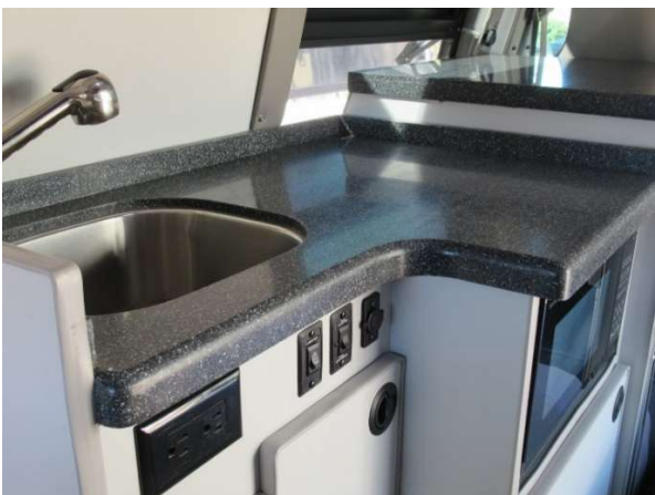
Sink with adjacent 20"Wx21"D work surface, under sink storage, and extra-long faucet hose.
