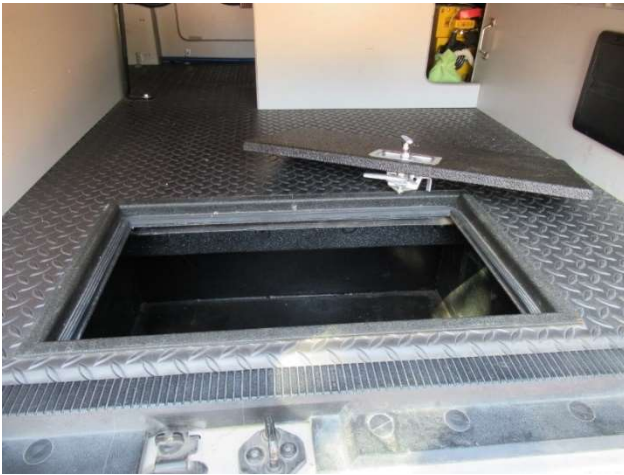
Rear under-floor lockable storage pit, 31x28x13.
