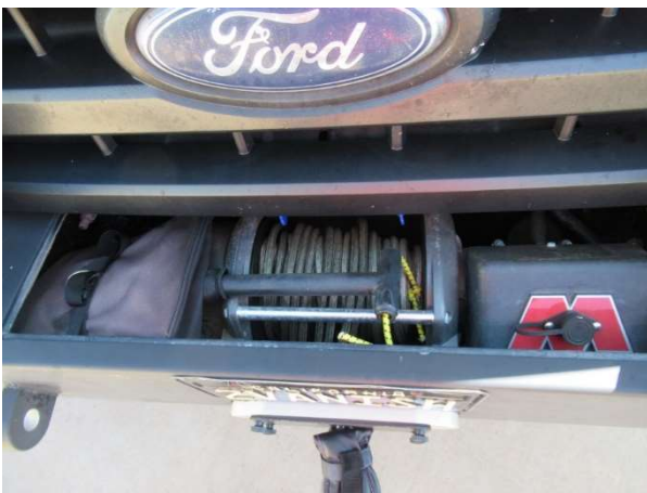
Front hatch with 12,000-pound Warn Winch with Dyneema cable, shovel, and Hi-Lift jack handle.
