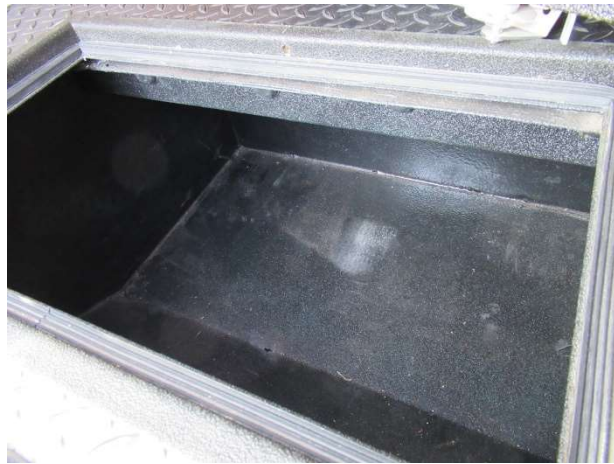
Interior rear storage: main compartment 40"Wx55"Dx13"H, and side cabinets 14"Wx36"Dx12"H.
