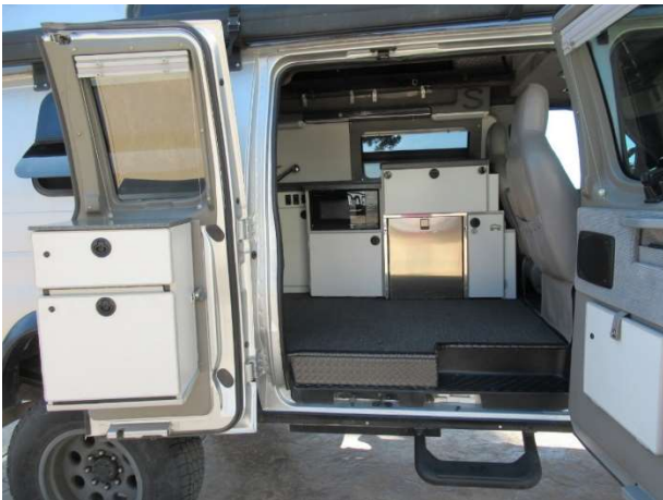
Door-mounted galley box, kitchen area with two-tier storage shelves, LED lights, heat reflective panel.
