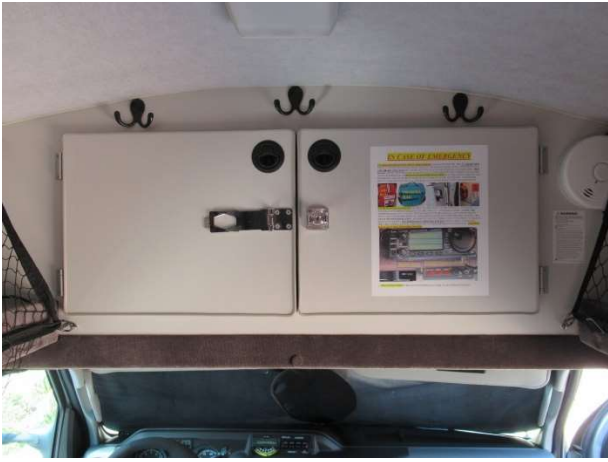
Lockable storage over front seats, 57x25x18, wedge shape. Insulated ceiling, with overhead air vent fan with cover, rain detecting.
