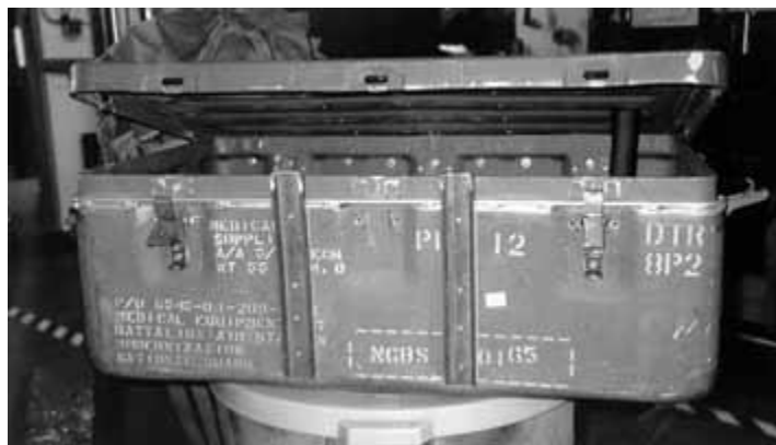
Figure 1—Surplus medical box modified to be bear-resistant. One side can be hinged or both sides can be secured with latches.
