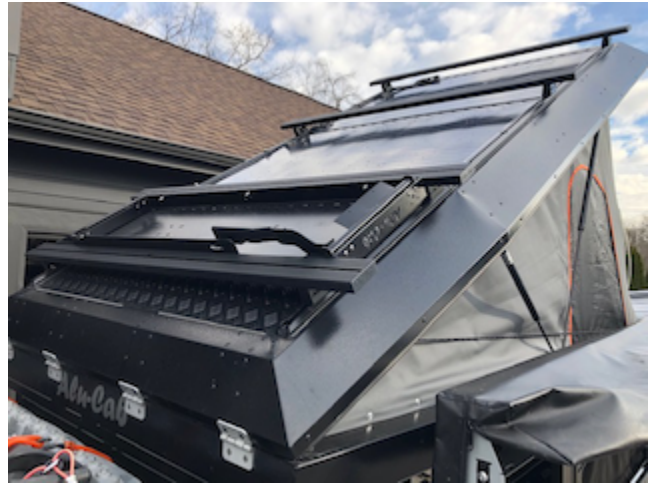
Roof bars, Maxtrax holder & 2x 105w solar panels
