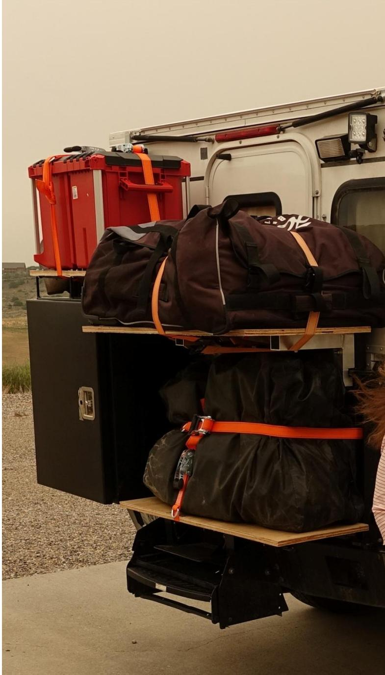
Cargo rack carrying pontoon boat equipment in a gear bag, inflatable kayak in a gear bag. Can carry paddle boards or other recreation equipment instead.
