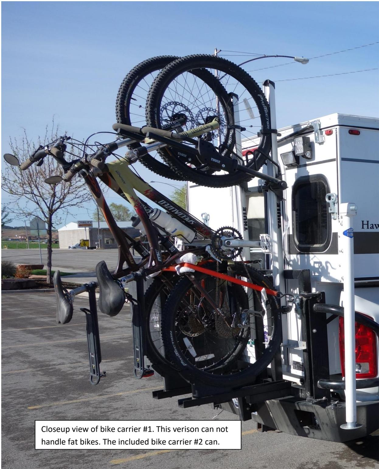
Closeup view of bike carrier #1. This version can not handle fat bikes. The included bike carrier #2 can.
