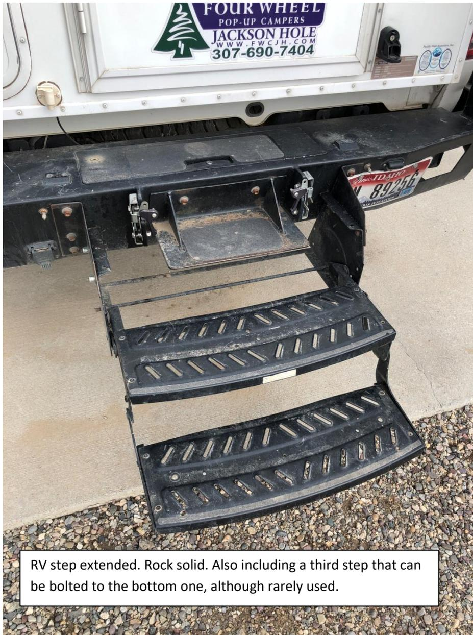
RV step extended. Rock solid. Also including a third step that can be bolted to the bottom one, although rarely used.
